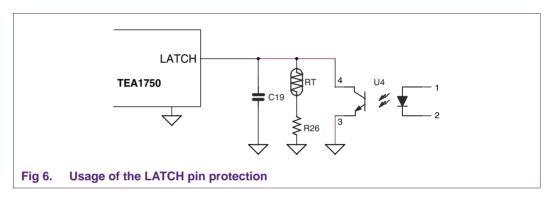
Latching on application over temperature occurs when the total resistance value of the NTC and its series resistor drops below the following:
