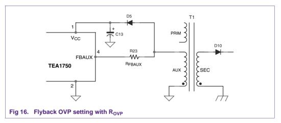
At a current  $I_{ovp(FBAUX)}$  of 300  $\,\mu A$  into the FBAUX pin, the IC detects an overvoltage. An internal integrator filters noise and voltage spikes. The output of the integrator is used as an input for an up-down counter. The counter has been added as an extra filter to prevent false OVP detection, which might occur during ESD or lightning events.
