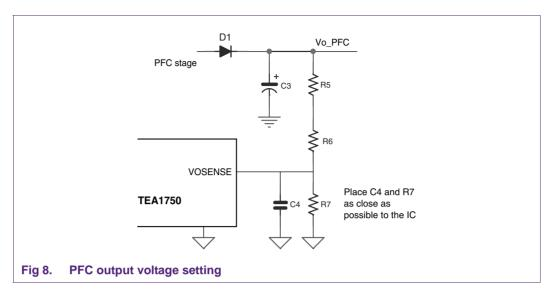
For low no-load input power two resistors of 4.7 M $\Omega$  (1%) can be used between the bulk elcap and the VOSENSE pin.
