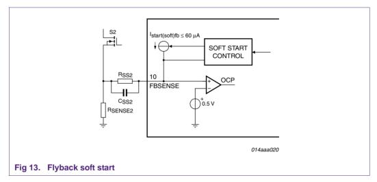
Rss2 must have a minimum value of 12 k $\Omega$  as specified. This to ensure that the voltage  $V_{\text{start(soft)PFC}}$  of 0.5 V is reached to enable start-up of the flyback. See Section 3.1 for start-up description.
